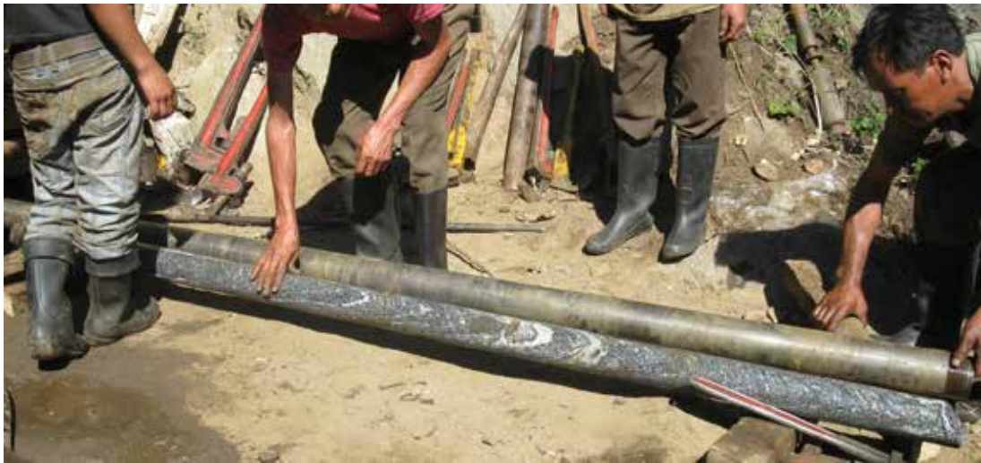
Picture 1 100% Core recovery in gneissic rock of Sela group, Tawang HEP, Arunachal Pradesh, India
