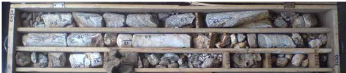
Picture 2 Poor core recovery in sheared gneissic rock of Sela Group, Tawang, A.P.
