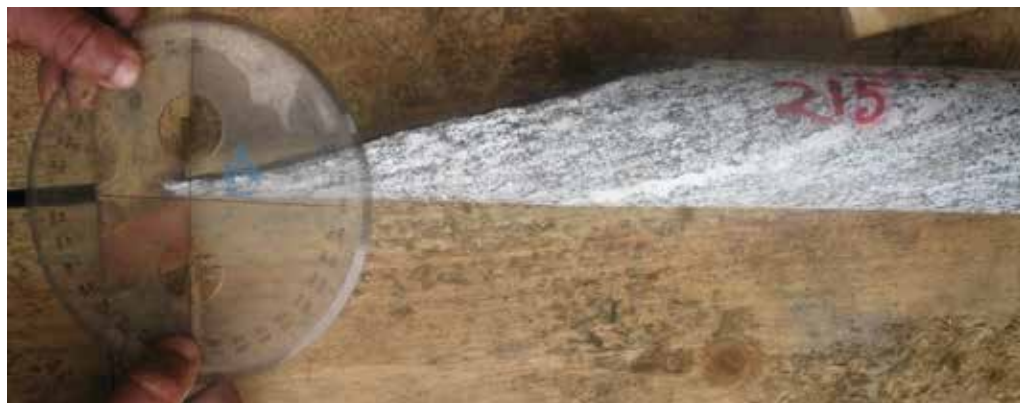
Picture 4 Precisely measured inclination of foliation in the core samples
